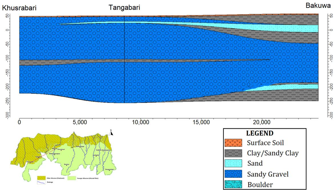
Fig 3.1.4 : Section of Khusrabari- Bakuwa Section
